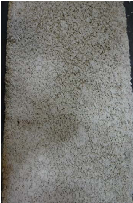
Hemp side exposed to test flame.
